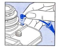
It is advisable to operate the rapid transport lever before inserting the flash bulb. Then
