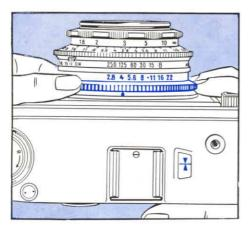
Turn the aperture setting ring to centre the pointer on the setting mark.
