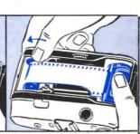
Open camera back by sliding shown Push locking button in direcdirection 2 catch by arrow. the
