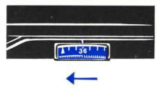
ting the scale to the green triangle between 36 and 1, for films with 20 exposures the green triangle between 25 and 20. The camera is ready for the first exposure after transporting the film to bring this number (i. e. 36 or 20) opposite the fixed setting mark (see illustration). The film counter indicates the number of exposures you still have left on the film.
