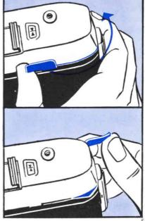
Your camera's readiness for instant action is largely increased by this rapid transport lever; this is a real advantage when taking a series of pictures. Very often split-second timing is needed to capture a tense or comical situation with the camera. If you line up horizontal subjects in the viewfinder with your right eye you need not even lower the camera to transport the film. You just move the lever with your right thumb and are always "in the picture".
